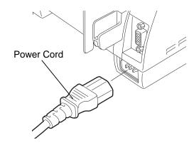
**3.** Plug the other end of the Power Cord into the ground outlet as shown in the figure below.
